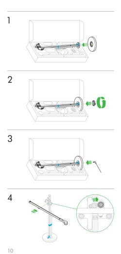
It is important that the light is assembled in the box as shown. Do not remove the transit tape until the light is fully assembled.
