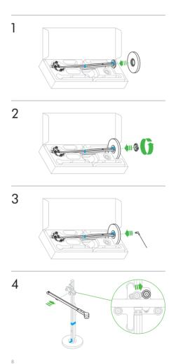
It is important that the light is assembled in the box as shown. Do not remove the transit tape until the light is fully assembled.
