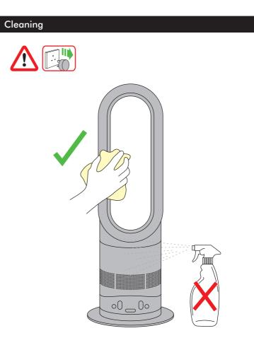
Unplug from the mains electricity supply. Allow to cool for 1 to 2 hours before cleaning if the heater has been in use. To clean, wipe with a dry or damp cloth. Do not use detergents or polishes.
