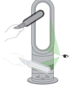
Ensure the heater is unplugged and has been allowed to cool. Look for blockages in the air inlet holes and in the small aperture inside the air loop amplifier. Use a soft brush to remove debris.
