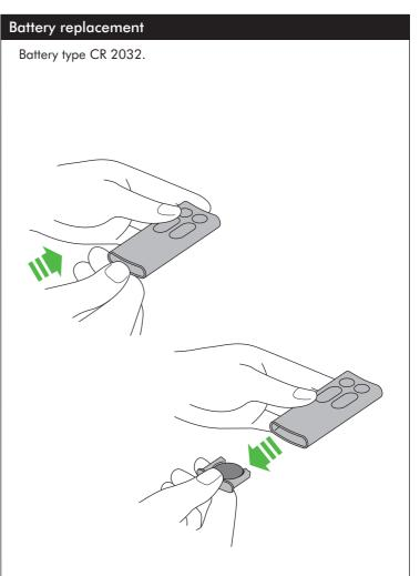
Press the end of the remote to release the battery.
