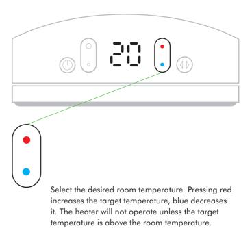
Cool air mode Press the blue thermostat control button to change the target temperature to 0°C. The power button light will change from red to blue. To adjust the airflow speed use the airflow speed control. To return to heating mode Press the red thermostat control button until the digital display
