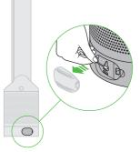
Clean the hatch every time the filter is replaced. Open the small hatch on the side of the appliance. Use a cotton bud to clean inside and remove any debris. This maintains sensor accuracy and ensures the continuing high performance of the appliance.
