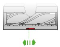
Your Torque Drive XL cleaner head has a slider control to adjust the suction of the cleaner head.
