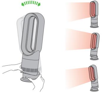
Carefully hold the base and the main body. Tilt the amplifier forward or backward for the required airflow angle.
