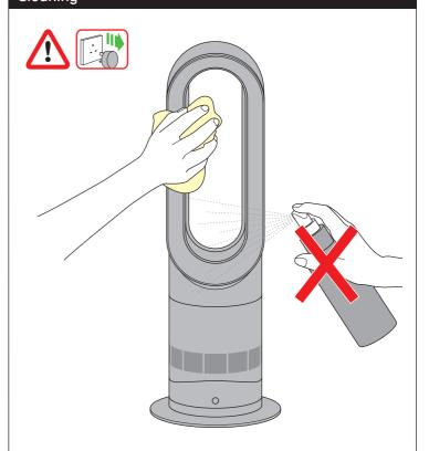
Unplug from the mains electricity supply. If the appliance has been in use, leave for 1 to 2 hours before cleaning to allow the appliance to cool completely. To clean, wipe with a dry or damp cloth. Do not use detergents or polishes.
