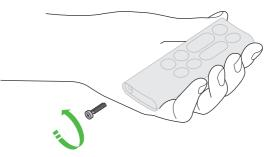
Unscrew the battery compartment on the remote control. Loosen the base and pull to remove the battery.
