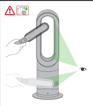
Ensure the appliance is unplugged. If the appliance has been in use, leave for 1 to 2 hours in order to allow the appliance to cool down completely. Look for blockages in the air inlet holes and in the small aperture inside the air loop amplifier. Use a soft brush to remove debris.
